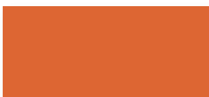
Sanodure Fast Bronze L 0.20 g/l Sanodal Red B3LW 0.25 g/l, T=40°C
